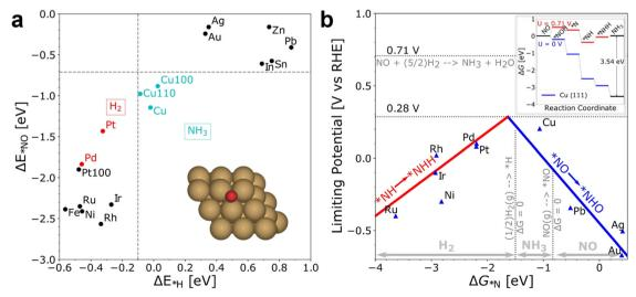
Fig. 3 (a) The adsorption energies of the intermediates  $\Delta E_{\mathrm{NO}}^*$  are plotted against  $\Delta E_{\mathrm{H}}^*$  on various metal surfaces. (b) The limiting potential volcano plot for NO reduction to NH<sub>3</sub> on various metal surfaces. Reproduced with permission from ref. 43 copyright 2021, Wiley-VCH.
