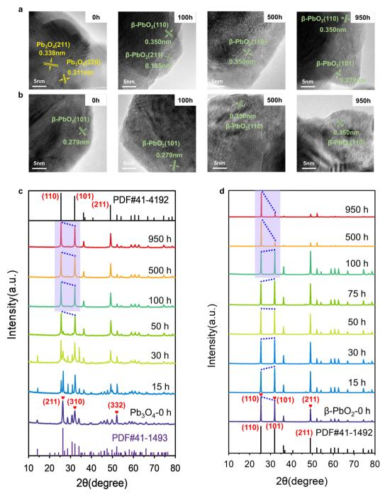
Fig. 2 Structural characterization of  $Pb_3O_4$  and  $\beta$ - $PbO_2$  in MEA under different EOP durations. (a and b) HRTEM images and (c and d) ex situ XRD patterns of Pb<sub>3</sub>O<sub>4</sub> and  $\beta$ -PbO<sub>2</sub> before and after EOP treatment in EOP electrolyzer at a high current of 1 A cm<sup>-2</sup>.
