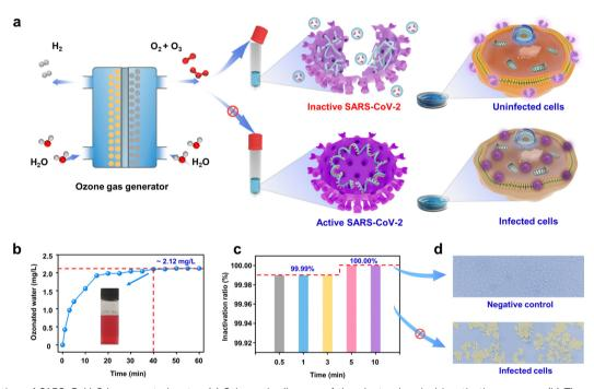
Fig. 5 Inactivation of SARS-CoV-2 by ozonated water. (a) Schematic diagram of the electrochemical inactivation process. (b) The concentration of ozonated water collected in 15 mL of normal saline under normal temperature and pressure (Inset: The qualitative result of ozonated water concentration). (c) SARS-CoV-2 inactivation ratio by ozonated water. (d) Microscopic pictures of negative control and infected cells by SARS-CoV-2 (400× magnification).
