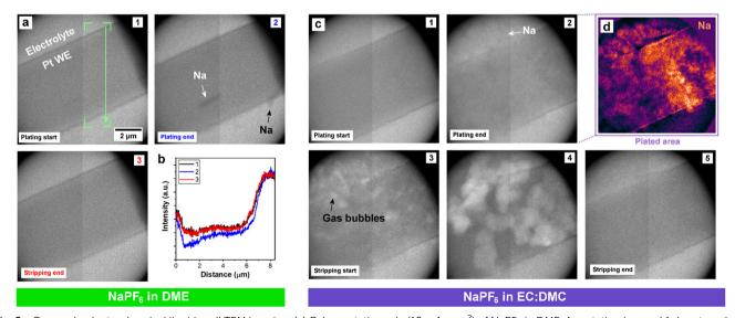
Fig. 2 Operando electrochemical liquid-cell TEM imaging. (a) Galvanostatic cycle (10 mA cm<sup>-2</sup>) of NaPF<sub>6</sub> in DME. Annotation in panel 1 denotes where box-averaged intensity profiles were acquired from each panel. (b) Intensity profiles extracted from panels 1 to 3. (c) Galvanostatic cycle ( $10 \text{ mA cm}^{-2}$ ) of NaPF<sub>6</sub> in EC:DMC. (d) False-color look-up table of panel 2 following background subtraction, highlighting Na deposition.
