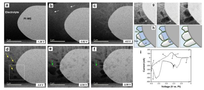
Fig. 3 Operando electrochemical HAADF-STEM imaging of bubble formation from 1 M NaPF<sub>6</sub> in EC:DMC with 10% FEC. (a-f) Liquid-cell STEM timeseries of cyclic voltammetry cycling showing Na plating and stripping. (g) Magnified views showing bubble formation during stripping. (h) Illustrations corresponding to (g). (i) Cyclic voltammetry profile corresponding to panels (a-f).
