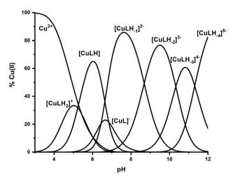
Fig. 1 Species distribution diagram of the system Cu(II)-Ac-GS(P) TENLKH-NH<sub>2</sub> at a molar ratio of 1:1.2 (C=2 mM).
