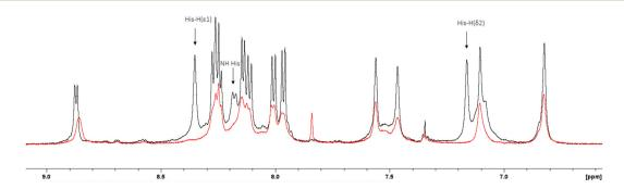
Fig. 4 Superposition of the  $^{1}$ H-NMR spectra (aromatic region) of the peptide R1P in the presence (red trace) and absence (black trace) of 0.05 eq. of Cu(II) ( $C_{peptide} = 2 \text{ mM}$ , H<sub>2</sub>O: D<sub>2</sub>O 9:1, v/v, pH = 6). The most affected resonances have been indicated by arrows.
