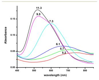
Fig. 8 Visible absorption spectra of the solutions of Cu(II) and R1 (Cu (II): R1 = 1:1.2, T = 298 K, I = 0.1 (KNO<sub>3</sub>)), recorded at the indicated pH values.
