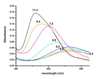
Fig. 2 Visible absorption spectra of the solutions of Cu(II) and R1P  $(Cu(II): R1P = 1: 1.2, T = 298 \text{ K}, I = 0.1 (KNO_3)), recorded at the indicated$ pH values
