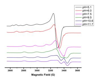
Fig. 9 EPR spectra of the Cu(II)-R1 system in a molar ratio of 1:1.2 at various pH values.
