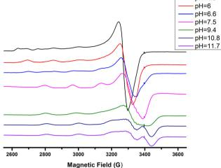
Fig. 3 EPR spectra of the Cu( $\pi$ )-R1P system in a molar ratio of 1:1.2 at various pH values.
