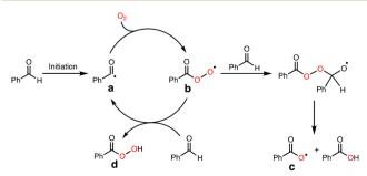
Scheme 3 Autoxidation mechanism of benzaldehyde.
