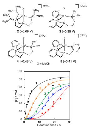
Fig. 3 Time courses of product formation in the oxidation of cyclohexane (2.0 M) catalysed by Cu<sup>II</sup>-complexes (1-5, 0.2 mM) with PhCHO (0.2 M) in  $CH_3CN/CH_2Cl_2$  (v/v = 3/2) at 40 °C under  $O_2$ . [P] = [A] + [K] + [L] + [CyCl]. Reduction potentials of the Cu<sup>II</sup>-complexes (vs. Fc/Fc<sup>+</sup> in acetonitrile) are shown in parentheses. The cyclic voltammograms of the Cu<sup>II</sup>-complexes are presented in Fig. S2.†
