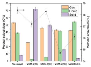
Fig. 2 The methane conversion and product selectivities of UZSM-5. and HZSM-5 catalysts with various SiO<sub>2</sub>/Al<sub>2</sub>O<sub>3</sub> ratios.
