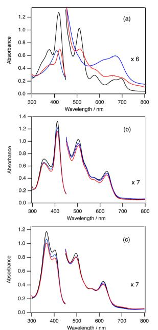
Fig. 3 Absorption spectral changes in the catalytic cyclohexane oxidation reactions of 2-Cl (a), 3-Cl (b), and 5-Cl (c) with mCPBA at 20 °C. Black line: before addition of mCPBA, blue line: immediately after the addition of mCPBA, red line; after 300 s.
