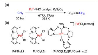
Fig. 1 (a) A schematic representation of conversion of methane to MeTFA; (b) structures of Pd<sup>II</sup>Br<sub>2</sub>L1, Pd<sup>II</sup>Br<sub>2</sub>L1 and [Pd<sup>II</sup>Cl(L3)<sub>2</sub>] [Pd<sup>II</sup>Cl<sub>3</sub>(dmso)] as catalysts.<sup>20</sup>
