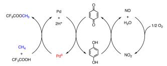
Scheme 3 Proposed reaction mechanism of a Pd<sup>II</sup>/Q/NO<sub>2</sub>/O<sub>2</sub> system to oxidize CH<sub>4</sub> in CF<sub>3</sub>COOH.<sup>21</sup>
