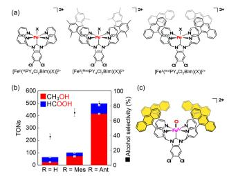
Fig. 6 (a) Schematic representations of  $[Fe^{II}(^{R}PY_{4}Cl_{2}BIm)(X)]^{2+}$  (R = H, Mes, Ant, X: OH<sub>2</sub>, OD<sub>2</sub>, NCCH<sub>3</sub> or NCC<sub>6</sub>H<sub>5</sub>). (b) Comparison of TONs and alcohol selectivity among the three catalysts. (c) Schematic representation of active species for methane oxidation by  $[Fe^{II}(^{Ant}PY_4Cl_2BIm)(OH_2)]^{2+}$  and  $Na_2S_2O_8$  in  $H_2O: CH_3CN = 95:5.62$
