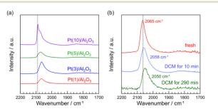
Fig. 5 FT-IR spectra of chemisorbed CO on Pt/Al<sub>2</sub>O<sub>3</sub> catalysts. (a) fresh Pt(1, 3, 5, and 10)/ $Al_2O_3$  and (b) fresh and spent Pt(1)/ $Al_2O_3$ . DCM reaction conditions: T = 600 °C, flow rate = 20 + 1 (CH<sub>4</sub> + H<sub>2</sub>) mL  $min^{-1}$ , catalyst mass = 0.10 g.
