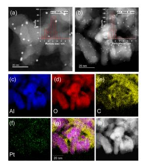
Fig. 2 HAADF-STEM images and particle size distribution of (a) fresh and (b) spent Pt(1)/Al<sub>2</sub>O<sub>3</sub>. EDX mapping images for (c) Al, (d) O, (e) C, (f) Pt, (g) overlay of (c-f), and (h) HAADF-STEM image of the spent catalyst. Spent catalyst: DCM was performed on Pt(1)/Al<sub>2</sub>O<sub>3</sub> for 5 h under CH<sub>4</sub>/H<sub>2</sub> (20/1).
