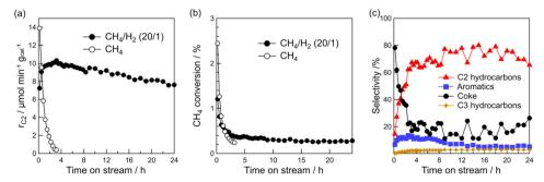
Fig. 6 Time course of (a) formation rate of C2 hydrocarbons, (b) methane conversion, and (c) product selectivity for DCM reaction. Catalyst: Pt(1)/  $Al_2O_3$ , T: 600 °C, flow rate: 20 (CH<sub>4</sub>) and 20 + 1 (CH<sub>4</sub> + H<sub>2</sub>) mL min<sup>-1</sup>, and catalyst mass: 0.10 g.
