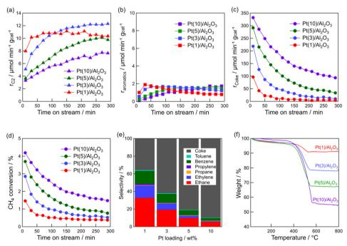
Fig. 3 Time course of formation rate of (a) C2 hydrocarbons, (b) aromatics, (c) coke, and (d) CH4 conversion for DCM reaction. (e) Product selectivity for DCM reaction. (f) TG profiles of the spent catalysts. Catalysts: Pt(1, 3, 5, and 10)/ $Al_2O_3$ , T: 600 °C, flow rate: 20 + 1 (CH<sub>4</sub> + H<sub>2</sub>) mL min<sup>-1</sup>, and catalyst mass: 0.10 g.
