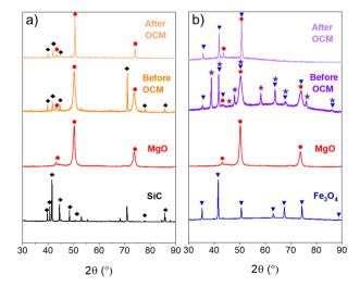
Fig. 3 X-ray diffraction patterns of a) SiC, MgO and SiC@MgO catalysts before and after OCM reaction under microwave heating (MW) and b) Fe<sub>3</sub>O<sub>4</sub>, MgO and Fe<sub>3</sub>O<sub>4</sub>@MgO catalysts before and after OCM under microwave heating (MW). SiC (♦), MgO (●), Fe<sub>3</sub>O<sub>4</sub> (▼) and  $Fe_2O_3$  ( $\star$ ).
