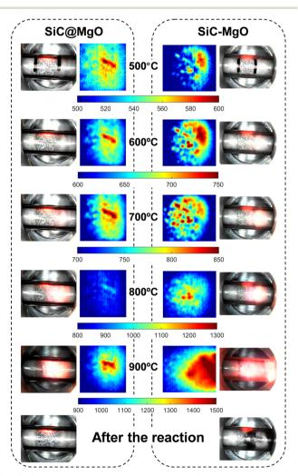
Fig. 6 Digital microscopy images and infrared thermography images during OCM under MW at different reaction temperatures for the SiC@MgO and SiC-MgO catalytic beds. The red light reflected on the reactor wall is the focusing light from the infrared temperature sensor. The gas flow is from the left to the right of the reactor tube.
