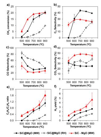
Fig. 4 a)  $CH_4$  conversion, b)  $C_2$  selectivity, c) CO selectivity, d)  $CO_2$ selectivity, e) C<sub>2</sub>H<sub>4</sub>/C<sub>2</sub>H<sub>6</sub> ratio and f) H<sub>2</sub> yield for SiC@MgO catalyst under microwave radiation (MW) and resistive heating (RH) conditions and SiC-MgO catalyst under microwave radiation (MW) conditions.
