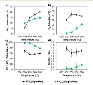
Fig. 7 a)  $CH_4$  conversion, b)  $C_2$  selectivity, c)  $CO + CO_2$  selectivity and d)  $CO/CO_2$  ratio for SiC@MgO and  $Fe_3O_4@MgO$  catalysts under microwave radiation (MW) conditions.
