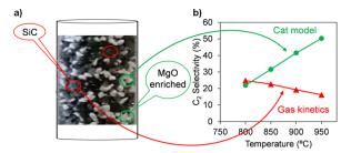
Fig. 5 a) Digital microscope image of the catalyst bed composed of SiC and MgO physically mixed particles, b) C2 selectivity calculated using the OCM gas-phase kinetic model reported by Chen et al.44 and the comprehensive kinetic model (accounting for the homogeneousheterogeneous nature of the OCM process) developed for the MgO catalyst, <sup>45</sup> at  $CH_4$ :  $O_2 = 4$ ,  $P_{CH_4} = 40\%$ , and  $X_{O_2} = 100\%$ .
