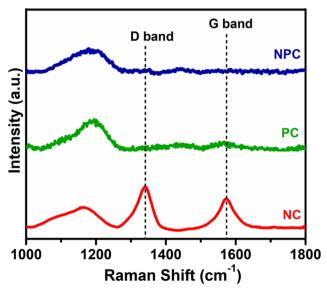
Fig. 11 Raman spectra of spent NC, PC and NPC catalysts.
