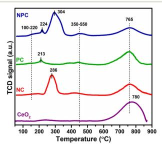
Fig. 5 H<sub>2</sub>-temperature programmed reduction pattern of undoped CeO<sub>2</sub>, NC, PC and NPC catalysts.
