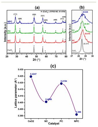
Fig. 1 Powder X-ray diffraction patterns of the reduced catalysts (a),  $2\theta$  shifting with respect to the (111) plane (b) and change in the lattice parameter corresponding to the (111) plane of the CeO2 lattice in NC, PC and NPC catalysts (c).
