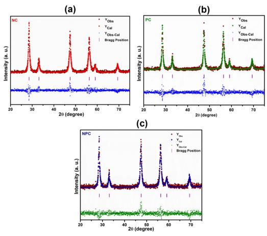
Fig. 2 Rietveld refinement XRD patterns of NC (a), PC (b), and NPC (c) catalysts. Difference between observed and calculated intensities (Yobs-cal), calculated intensity  $(Y_{cal})$  and observed intensity  $(Y_{obs})$ . Vertical lines indicate peak positions and differences.
