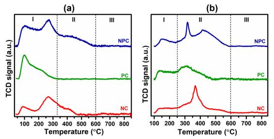
Fig. 12 Chemisorption properties of CeO<sub>2</sub>, NC, PC and NPC by CH<sub>4</sub>-TPD (a) and CO<sub>2</sub>-TPD (b).
