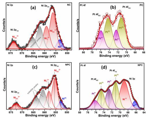
Fig. 7 XPS spectra: (a) Ni 2p and Pt 4f of the reduced NC catalyst, (b) Pt 4f of the reduced PC catalyst and (c and d) Ni 2p and Pt 4f of the reduced NPC catalyst.
