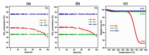
Fig. 14 (a and b) 100 h stability test over the prepared catalysts and (c) TGA graph of the spent catalysts after the TOS study (reaction conditions: GHSV – 50 000 mL  $h^{-1}$   $g^{-1}$ , temperature – 675 °C, feed ratio –  $CH_4: CO_2: N_2 - 1:1:5$ ).
