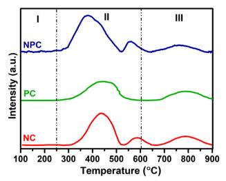
Fig. 8 O<sub>2</sub>-TPD patterns of fresh NC, PC and NPC catalysts.
