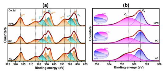
Fig. 6 XPS spectra of all the prepared catalysts: (a) Ce 3d and (b) O 1s.
