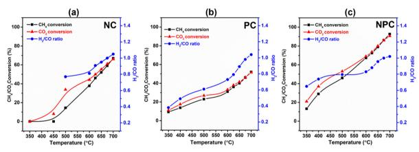
Fig. 13 Temperature effect on the conversion of CO<sub>2</sub>/CH<sub>4</sub> and H<sub>2</sub>/CO ratio over NC (a), PC (b), and NPC (c) catalysts (reaction conditions: GHSV -50 000 mL  $h^{-1}$   $g^{-1}$ , temperature – 350–700 °C, pressure – 1 atm, TOS – 6 h and feed ratio –  $CH_4$ :  $CO_2$ :  $N_2$  – 1:1:5).
