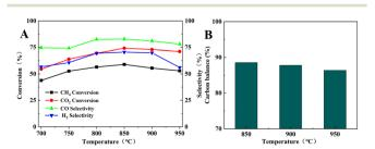
Fig. 9 (A) DRM catalytic performance of BCYF $_{0.10}$ -Ni powder, (B) carbon equilibrium (feed gas was 50 mL min<sup>-1</sup> CH<sub>4</sub> and 50 mL min<sup>-1</sup> CO<sub>2</sub>).
