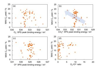
Fig. 1 Plots of maximum C2 yield against the three deconvoluted O1s XPS peaks assignable to (a)  $O_2^-$ , (b)  $CO_3^{2-}$ , and (c)  $O_3^{2-}$  species. (d) Plot of maximum  $C_2$  yield against  $O_2^-/O^{2-}$  ratio. Maximum  $C_2$  yield: the highest C2 yield value obtained with each catalyst in the experiment protocol.
