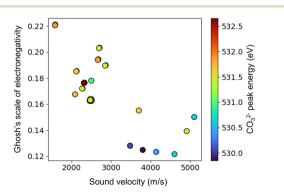
Fig. 3 Ghosh's scale of electronegativity (en\_ghosh) and sound velocity against CO<sub>3</sub><sup>2-</sup> peak energy.
