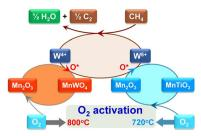
Fig. 6 Proposed catalytic cycle for OCM reaction mediated by the redox cycle Mn<sup>2+</sup> ↔ Mn<sup>3+</sup> over Mn-Na<sub>2</sub>WO<sub>4</sub>/Ti-MWW. Reprinted from ref. 36 with permission from The American Association for the Advancement of Science, copyright 2017.
