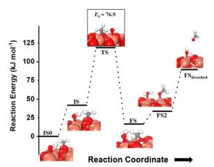
Fig. 13 The most stable initial state (ISO), reaction initial state for the second activation of methane (IS), transition state (TS), final states (FS and FS2), and desorbed state (FS<sub>desorbed</sub>) corresponding to the second activation of methane by surface hydroxides  $(OH)_{Cu \, site}^*$ . Activation energy barrier (kJ mol<sup>-1</sup>) is indicated. The color scheme is the same as in Fig. 2.
