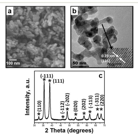
Fig. 15 Morphology and structure characterization of the as-synthesized CuO: a) SEM image depicting the nanopellet morphology, b) bright field TEM image with the HRTEM image insert for the nanopellets depicting lattice fringes corresponding to the (111) facet, and c) X-ray diffractograms of as-synthesized CuO with signature peaks of copper(II) oxide. 35 Copyright 2017 American Chemical Society.
