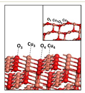
Fig. 1 The surface atomic arrangement on the CuO(111) facet showing the repeating arrangement of  $O_3$ - $Cu_3$ - $O_4$ - $Cu_4$  units, where the subscript denotes the coordination number of the respective atom. Peach and red balls represent copper (Cu) and oxygen (O) atoms,
