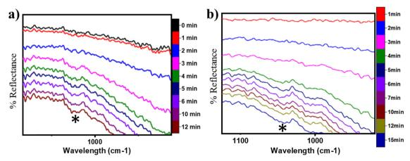
Fig. 16 DRIFT spectra at successive time intervals for the HC-O stretching region for (a) CH<sub>4</sub> oxidation on moist CuO at 300 °C and b) CH<sub>4</sub> oxidation on dry CuO at 300 °C. Symbols: (\*) 1050 cm<sup>-1</sup>.
