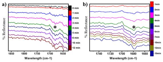
Fig. 17 DRIFT spectra at successive time intervals for the C=O stretching region in CH<sub>4</sub> oxidation at 300 °C under a) moist and b) dry conditions. (\*) is 1680 cm<sup>-1</sup>.
