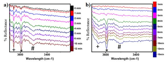
Fig. 18 DRIFT spectra at successive time intervals for the O-H stretching region for (a) CH<sub>4</sub> oxidation on moist CuO at 300 °C and b) CH<sub>4</sub> oxidation on dry CuO at 300 °C. Symbols: (\*) 3595 cm<sup>-1</sup>, (+) 3650 cm<sup>-1</sup>, (#) 3500 cm<sup>-1</sup>.
