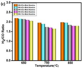
Fig. 5 Effect of temperature over the catalyst compositions at 10 L g<sup>-1</sup> h<sup>-1</sup> WHSV and at atmospheric pressure (a) CH<sub>4</sub> conversion (b) CO<sub>2</sub> conversion (c) H<sub>2</sub>/CO ratio. Prior to the activity study, the catalyst was reduced at 850 °C with 20% H<sub>2</sub>/N<sub>2</sub>.
