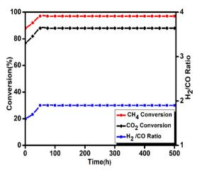
Fig. 8 Effect of time on stream for 5Ni-5Co-mod alumina at 850 °C with WHSV 10 L q<sup>-1</sup> h<sup>-1</sup> at atmospheric pressure. Prior to the activity study, the catalyst was reduced at 850 °C with 20% H<sub>2</sub>/N<sub>2</sub>.
