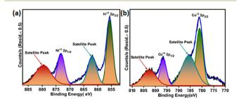
Fig. 3 XPS spectra for (a) Ni 2p and (b) Co 2p in 5Ni-5Co-mod
