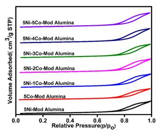
Fig. 1 N<sub>2</sub> adsorption-desorption isotherm profile of the freshly synthesized catalysts.
