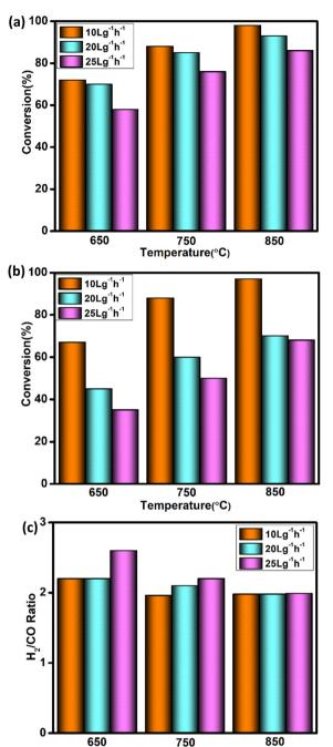
Fig. 6 Effect of space velocity and temperature on the catalytic activity under atmospheric pressure (a) CH<sub>4</sub> conversion (b) CO<sub>2</sub> conversion (c) H<sub>2</sub>/CO ratio of 5Ni-5Co-mod alumina. Prior to the activity study, the catalyst was reduced at 850 °C with 20% H<sub>2</sub>/N<sub>2</sub>.
