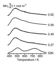
Fig. 5 NH<sub>3</sub> TPD profile of unloaded MFI(52N) and Co/MFI(52N). The samples were treated in an N2 flow at 773 K prior to the TPD measurement. The numbers indicate the loading of Co (mmol g<sup>-1</sup>).
