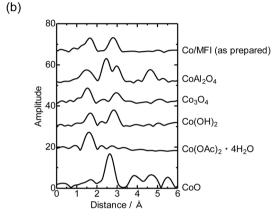
Fig. 1 Co K-edge (a) XANES and (b) EXAFS-FT of Co/MFI(52N) (Co: 0.5 mmol q<sup>-1</sup>) and reference compounds measured at 298 K. Fourier transform range: 3-13 Å<sup>-1</sup>.
