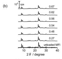
Fig. 6 XRD patterns of Co-unloaded MFI(52N) and Co/MFI(52N). (a) The as-prepared and (b) 773 K-treated samples. The numbers indicate the Co loading (mmol  $g^{-1}$ ).
