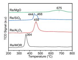
Fig. 2 TPR profiles of Re catalysts.
