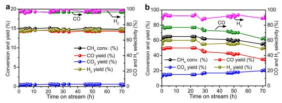
Fig. 4 Durability tests of Re/MOR. (a) CH<sub>4</sub>: O<sub>2</sub>: N<sub>2</sub> = 50:4:46. (b) CH<sub>4</sub>: O<sub>2</sub>: N<sub>2</sub> = 8:4:88. Conditions: 600 °C, SV of 12 000 mL g<sup>-1</sup> h<sup>-1</sup>.
