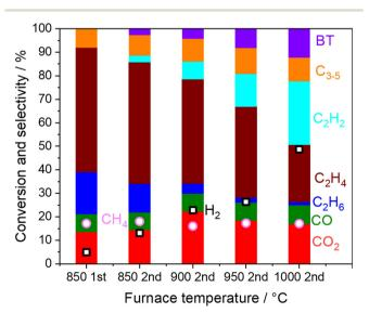
Fig. 3 Product distribution and CH<sub>4</sub> conversion from the outlets of the first and the second reactor. Inlet gas; CH<sub>4</sub> 10 kPa, O<sub>2</sub> 1.4 kPa, H<sub>2</sub>O 1.7 kPa, total pressure 101 kPa, Ar balance, 40 mL  $\min^{-1}$ . The first reactor; 800 mg of 5 wt% Na<sub>2</sub>WO<sub>4</sub>/SiO<sub>2</sub> at 850 °C. The second reactor; without catalysts at 850-1000 °C. O2 is depleted under all the conditions.
