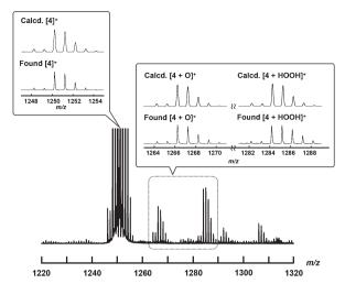
Fig. 6 ESI-TOF MS spectrum of 4<sup>+</sup>·I<sub>3</sub><sup>-</sup> in an aqueous CH<sub>3</sub>CN solution containing excess amount of H2O2 at room temperature (the detail of the experimental procedure is shown in the Experimental section). Insets: Comparison of calculated (top) and experimental (bottom) isotopic distribution patterns of molecular peaks assignable to [4]<sup>+</sup>, [4 + O]<sup>+</sup>, and [4 + HOOH]<sup>+</sup>.
