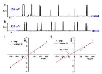
Fig. 3 Current traces of 2 at (a) 150 mV and (b) 120 mV in symmetrical KCl bath solutions (cis/trans = 1.0 M/1.0 M). I-V plots under (c) symmetrical (cis/trans = 1.0 M/1.0 M) and (d) asymmetric (cis/trans = 1.0 M/0.25 M) KCl bath solutions. Reversal potential  $V_r = -9.37 \text{ mV}$ . <sup>9a,13</sup> The final concentration of 2 is  $1.0 \mu M$ .
