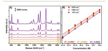
Fig. 6 SERS spectra of (A) R6G on ESD by focusing ion funnel substrate from  $10^{-4}$  M to  $10^{-10}$  M and (B) the Raman signal intensity of R6G at 612, 1362, and 1510 cm<sup>-1</sup> peaks as a function of molecular concentration (log scale).
