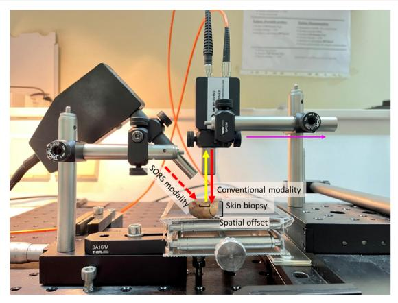
Fig. 2 Raman setup in the conventional (excitation indicated with red solid arrow) and SORS (excitation with red dashed arrow) configurations. The yellow solid arrow indicates the collection probe. A translational XY stage was used to move the collection (magenta arrow) away from the external excitation path and a vertical Z stage to adjust the working distance of the conventional/collection probe.
