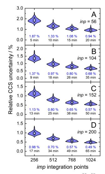
Fig. 5 Distributions of relative CCS uncertainties,  $\sigma_{\rm Cl}(\Omega^{(1.1)})/\Omega^{(1.1)}$ , for the validation set (N=50) for different combinations of velocity sample points (inp) and orientation/impact parameter sample points (imp). Blue numbers below each distribution correspond to mean relative CCS uncertainties and black numbers to average computing time.
