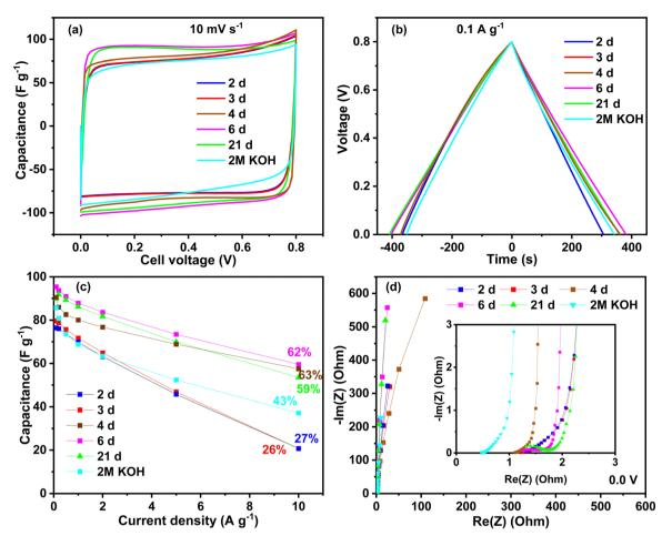
Fig. 5 Electrochemical performance of activated carbon symmetric capacitors using chitosan-KOH gel electrolyte obtained by different ageing times of the solution. (a) Cyclic voltammetry at 10 mV s $^{-1}$  (b) galvanostatic charge discharge at 0.1 A g $^{-1}$ . (c) Rate capability up to 10 A g $^{-1}$ . (d) Electrochemical impedance spectroscopy at 0.0 V (inset: EIS at high frequency).
