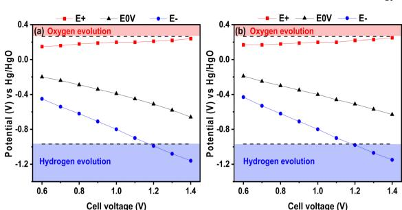
Fig. 6 Potential over cell voltage from 0.6 to 1.4 V in a 3-electrode cell using (a) liquid 2 M KOH and (b) chitosan-KOH gel electrolyte as electrolytes.
