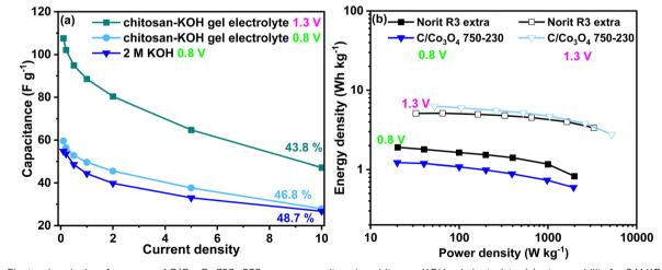
Fig. 10 Electrochemical performance of  $C/Co_3O_4$  750–230 nanocomposite using chitosan–KOH gel electrolyte: (a) rate capability for 2 M KOH at 0.8 V and for chitosan–KOH gel electrolyte at 0.8 and 1.3 V, (b) Ragone diagram of  $C/Co_3O_4$  750–230 nanocomposite and Norit R3 extra using 2 M KOH at 0.8 V and chitosan–KOH gel electrolyte at 1.3 V.
