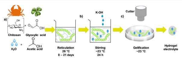
Fig. 1 Schematic representation of the preparation of the chitosan-KOH gel electrolyte including the following steps: (a) polymer host + solvent solution, (b) addition of KOH aqueous electrolyte, (c) solution casting in a petri dish.
