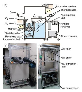
Fig. 2 Equipment for submerged comminution of LIBs in lime water under N<sub>2</sub> flow. (a) Schematic illustration. Photographs of (b) glove box with lime-water tank and (c) setup for N<sub>2</sub> gas supply (maximum flow rate 22.0 L min<sup>-1</sup> @ 99.9% N<sub>2</sub>, 56.4 L min<sup>-1</sup> @ 99% N<sub>2</sub>).
