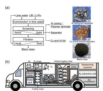
Fig. 4 Overview of the recycling process of LIBs utilizing the submerged comminution. (a) Flow chart of deactivation and physical sorting process for spent LIBs by submerged comminution with lime water. (b) Schematic illustration of processing vehicle for the end-of-life LIBs.
