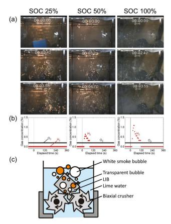
Fig. 3 Observation and analysis of the submerged comminution. (a) Photographs of cell batteries being comminuted. (b) Concentration trend of hydrogen above the water surface and oxygen in the glove box. (c) Schematic illustration of the comminution in lime water for the higher
