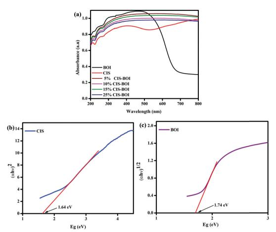
(a) UV absorbance spectra of pristine BOI, CIS and varying weight% CIS-BOI composites; Tauc plots of (b) pristine CIS and (c) pristine BOI.
