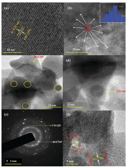
Fig. 3 HRTEM of the (a) fringe pattern of the CIS QDs, (b) image and size-distribution curve of the CIS QDs (inset), (c and d) deposition of the CIS QDs on the BOI MPs in the 15% CIS-BOI composite, (e) the SAED image of the 15% CIS-BOI composite, and (f) the fringe pattern of the 15% CIS-BOI composite.
