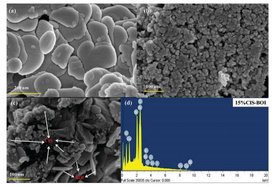
Fig. 2 FESEM images of (a) pristine BOI, (b) pristine CIS, and (c) the 15% CIS-BOI composite, and (d) the EDX spectrum of 15% CIS-BOI.
