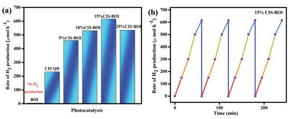
Fig. 11 (a) Rate of H<sub>2</sub> production of pristine CIS, BOI and CIS-BOI composites with varying wt% of CIS; (b) reusability of the 15% CIS-BOI composite.
