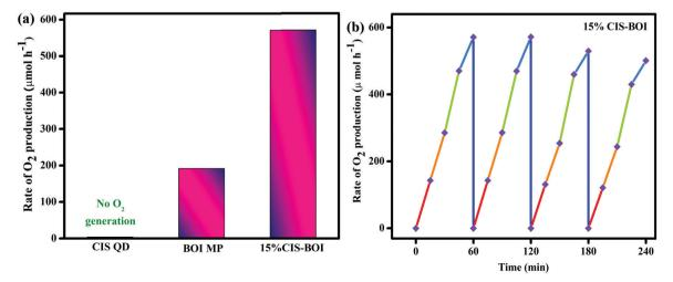
Fig. 12 (a) Rate of O<sub>2</sub> production of pristine CIS, BOI and the 15% CIS-BOI hybrid; (b) reusability of the 15% CIS-BOI hybrid.
