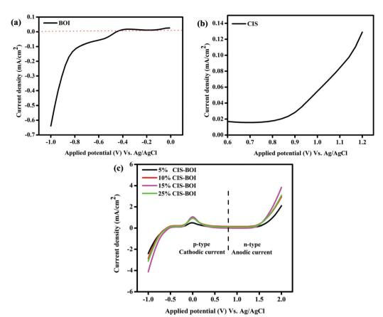
LSV plots of (a) pristine BOI, (b) pristine CIS, and (c) CIS-BOI composites with varying wt% of CIS
