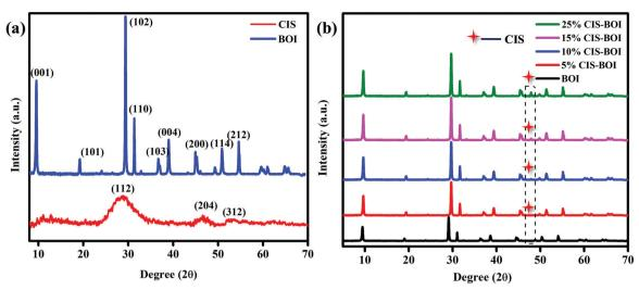
Fig. 1 PXRD patterns of (a) pristine CIS and BOI and (b) the CIS-BOI composites with varying CIS content.
