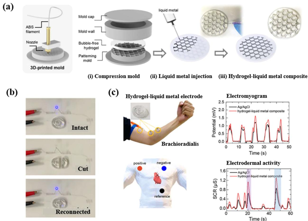
Fig. 7 The hydrogel-LM composite was applied in a multinodular sensor system.<sup>116</sup> (a) Schematic illustration of manufacturing the hydrogel-LM composite by 3D printing technology. (b) The self-healing capacity of the hydrogel-LM composite was evaluated using an LED. (c) Hydrogel-LM composite-based electrodes were used to detect bio-signals. Copyright 2020 American Chemical Society.
