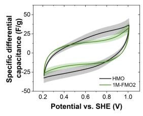
Fig. 2 Averaged specific differential capacitance of 2D  $MnO_x$  nanosheets (HMO) and nanocone-rich  $Fe_xMn_{1-x}O_2$  (1M-FMO2) sample. The standard deviation was used to obtain the error bar reported in the
