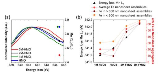
Fig. 8 (a) Left-YAxis: EELS Mn  $L_3$  peaks of HMO, 1M-HMO, 2M-HMO and 3M-HMO. Right-Yaxis: corresponding Mn  $I(L_3)/(L_2)$  values. (b) Trends of oxidation state of xM-HMO (Left-Yaxis) and Fe introduced by galvanic exchange reaction (right-Yaxis) for xM-FMO2.
