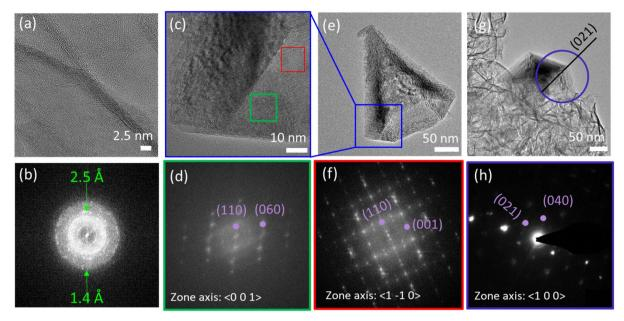
Fig. 6 (a and b) HRTEM micrograph and corresponding FFT pattern of a HMO nanosheet. (c-f) HRTEM micrographs and FFT patterns corresponding to two facets of a FMO2 nanocone. (g and h) TEM micrograph and corresponding SAED pattern of a FMO2 nanocone.
