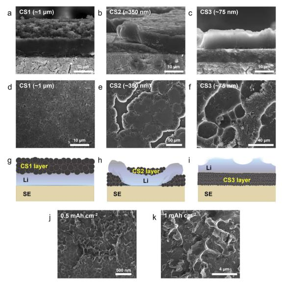
Fig. 2 (a-c) Cross-sectional and (d-f) top-view SEM images and (q-i) schematic illustrations of the Li in CS composite anodes deposited to a capacity of 3 mA h cm<sup>-2</sup>. (a, d, and g) for CS1, (b, e, and h) for CS2, and (c, f, and i) for CS3. Top-view SEM images of Li deposits on the CS3 composite anode at capacities of (j) 0.5 and (k) 1 mA h cm<sup>-2</sup>
