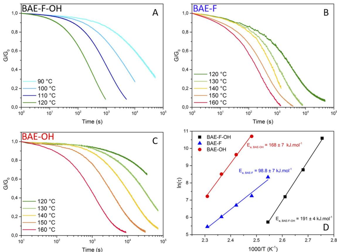
Fig. 4 Normalized stress-relaxation curves at different temperatures for a 1% strain (A) for BAE-F-OH, (B) for BAE-F and (C) for BAE-O. (D) Fitting of the relaxation time ( $\tau$ ) vs. temperature data by the Arrhenius equation for BAE-F-OH (black squares), BAE-F (blue triangle) and BAE-OH (red circles).
