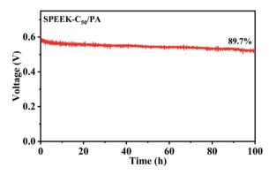
Fig. 7 long-term durability test of the DMFC with the SPEEK-C $_{50}/PA$  membrane under a current density of 300 mA cm $^{-2}$  with 2 M MeOH at 80  $^{\circ}\text{C}.$
