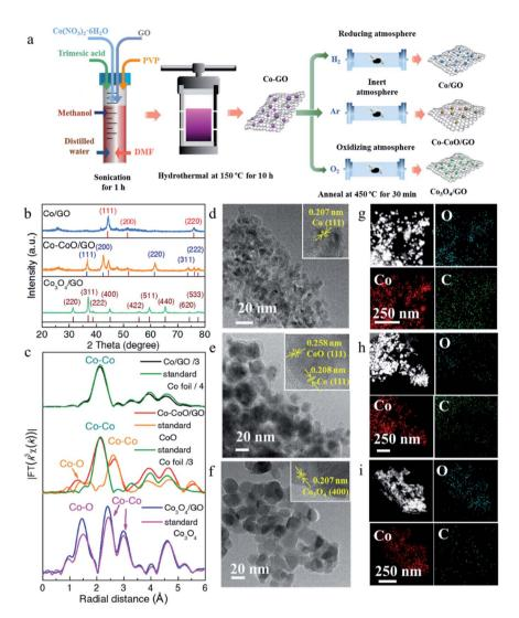
Fig. 1 (a) Schematic illustration of the synthesis of Co/GO, Co-CoO/GO and  $Co_3O_4/GO$ . (b) XRD patterns of Co/GO, Co-CoO/GO and  $Co_3O_4/GO$ . GO. (c) The corresponding  $k^3$ -weighted FT spectra of Co/GO, Co–CoO/GO and Co<sub>3</sub>O<sub>4</sub>/GO. The TEM images of Co/GO (d), Co–CoO/GO (e) and Co<sub>3</sub>O<sub>4</sub>/GO (f), and the insets display the HRTEM images of Co-based catalysts. EDS mapping images of Co/GO (g), Co-CoO/GO (h) and Co3O4/GO (i).
