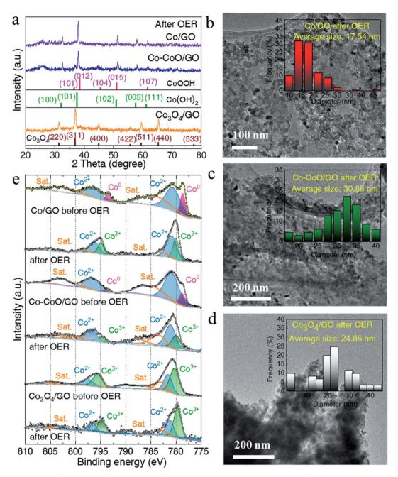
Fig. 3 (a) XRD patterns of Co/GO, Co-CoO/GO and Co<sub>3</sub>O<sub>4</sub>/GO after OER tests. The TEM images of Co/GO (b), Co-CoO/GO (c) and Co<sub>3</sub>O<sub>4</sub>/GO (d) after OER tests. The inset is the corresponding size distribution. (e) Co 2p XPS spectra of Co/GO, Co-CoO/GO and Co<sub>3</sub>O<sub>4</sub>/GO before and after OER tests.
