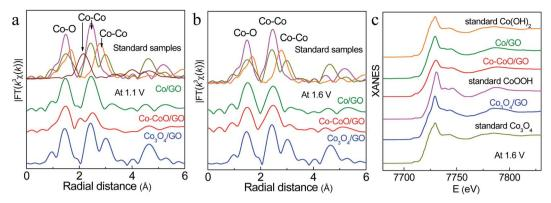
Fig. 4 In situ  $k^3$ -weighted FT spectra of Co–CoO/GO, Co/GO and Co $_3$ O $_4$ /GO at 1.1 V (a) and 1.6 V (b). In situ Co K-edge XANES spectra of Co–CoO/GO, Co/GO and Co $_3$ O $_4$ /GO at 1.6 V (c). The pink, orange, dark yellow and wine red lines represent the standard samples CoOOH, Co(OH) $_2$ , Co $_3$ O $_4$  and Co foil, respectively.
