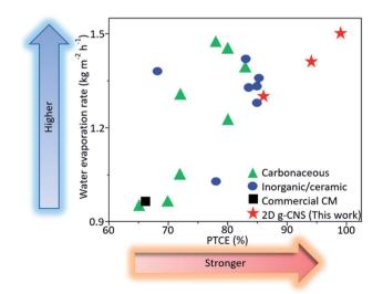
Fig. 5 Comparison of solar vapor generation performances of 2D g-CNS solar evaporators with previously reported solar evaporators under one-sun illumination (see details in Table S1, ESI†).
