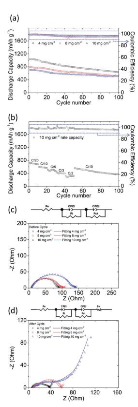
Fig. 3 Electrochemical analysis results of high-sulfur-loading cells: (a) cyclability; (b) rate performance at a sulfur loading of 10 mg cm<sup>-2</sup>; and EIS images (c) before and (d) after cycling
