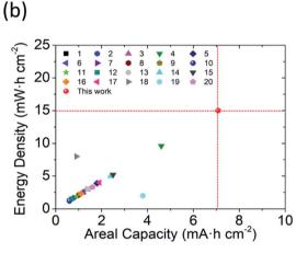
Fig. 5 Comparison of the cell-design parameters and cell-electrochemical performances of lithium-sulfur batteries with the PMMAbased GPE and other GPEs: (a) sulfur loading (mg cm<sup>-2</sup>) and content (wt%) and (b) areal capacity (mA h cm<sup>-2</sup>) and energy density (mW h cm<sup>-2</sup>) based on the whole electrode
