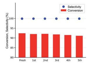
Fig. 7 Reusability test of the MOF-801(D) catalyst (ECH 19.2 mmol, catalysts 0.6 mol%, TBABr 0.5 mol%, 80 °C, 15 h, 0.1 MPa, semi-batch).
