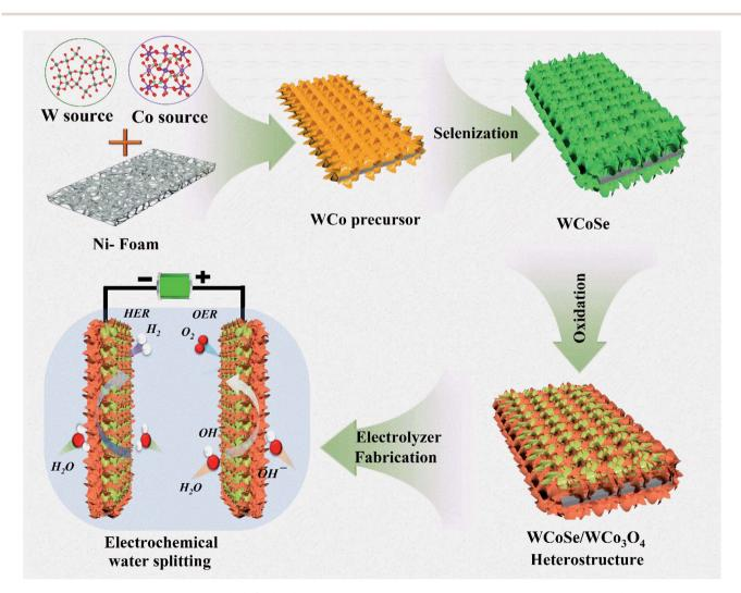
Scheme 1 Design and fabrication of the  $WCoSe/WCo_3O_4$  heterostructure *via* controlled surface atomic configuration for the alkaline medium electrochemical water-electrolyzer.
