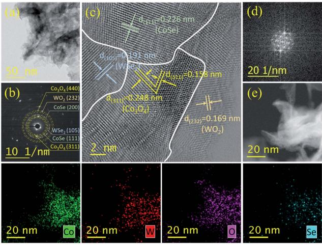
Fig. 2 Intrinsic morphology of the WCoSe/WCo $_3$ O $_4$  heterostructure. (a) TEM, (b) corresponding SAED, (c) HR-TEM, (d) FFT, and (e) STEM and STEM-EDS color mapping with the distribution of Co, W, O, and Se elements.
