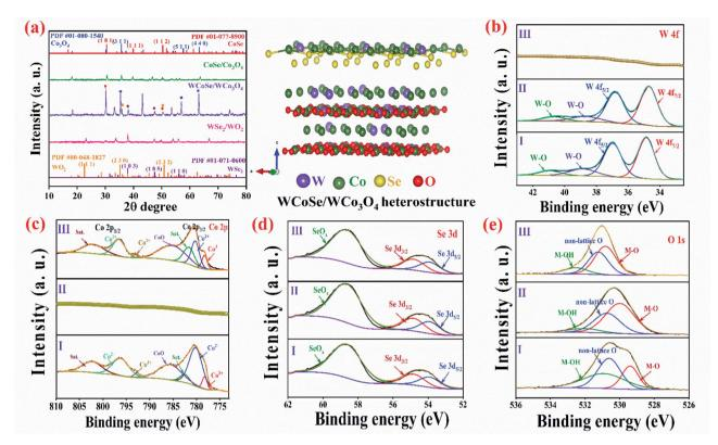
Fig. 3 (a) XRD patterns for the as-synthesized materials and structural alignments of the WCoSe/WCo<sub>3</sub>O<sub>4</sub> heterostructure. XPS spectra of (b) W 4f, (c) Co 2p, (d) Se 3d, and (e) O 1s present in the WCoSe/WCo<sub>3</sub>O<sub>4</sub> heterostructure.
