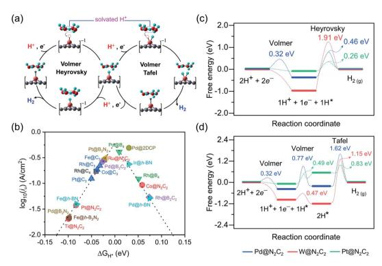
Fig. 3 (a) Schematic representation for the mechanisms and reaction pathways of electrocatalytic reaction cycles over different proposed 2D surfaces. (b) HER volcano plot for the promising electrocatalysts. The exchange current density plotted versus the calculated free energy of Hadsorption. Free energy diagram for the (c) Volmer-Heyrovsky and (d) Volmer-Tafel route on  $Pd@N_2C_2$  (blue color),  $W@N_2C_2$  (red color) and Pt@N2C2 (green color) surfaces.
