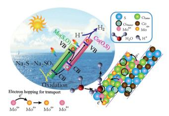
Fig. 15 Mechanism diagram of photocatalytic hydrogen production in the presence of the MoCoOS catalyst.
