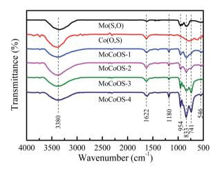
Fig. 3 FTIR spectra of Mo(S,O), Co(O,S), and MoCoOS prepared with different amounts of CoCl $_2\cdot$ 6H $_2$ O.
