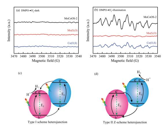
Fig. 14 EPR spectra of (a) DMPO-'O and (b) DMPO-'O<sub>2</sub>- for Mo(S,O), Co(O,S), and MoCoOS catalysts under darkness and illumination for 10 min. (c and d) The two types of heterojunction.
