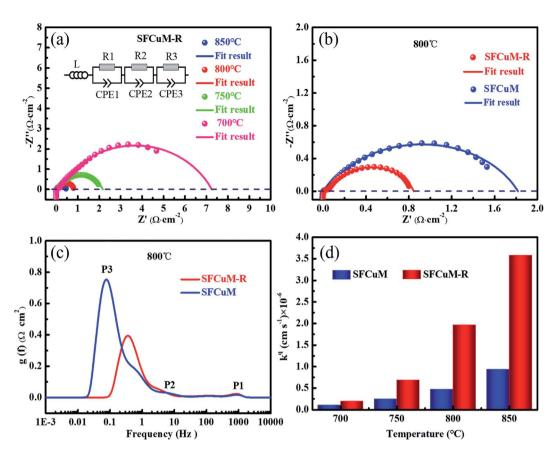
Fig. 7 (a) EIS of LSGM electrolyte-supported symmetrical cells with the configuration SFCuM-R/LDC/LSGM/LDC/SFCuM-R under a 1:1 CO–CO<sub>2</sub> atmosphere at different operating temperatures; (b) comparison of the EIS spectra using different electrodes at 800 °C; (c) assessment of the DRT spectrum at 800 °C; (d) calculated  $k^q$  of the different electrodes.
