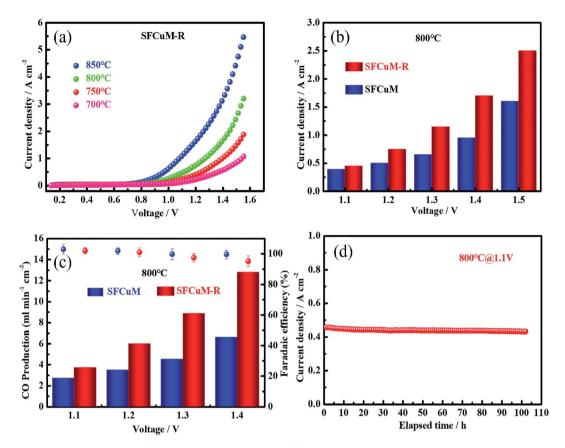
Fig. 8 (a) Single-cell current density with SFCuM-R as the fuel electrodes; (b) current density comparison of the cell with various fuel electrodes; (c) production of CO and faradaic efficiency; (d) long-term electrochemical stability during CO<sub>2</sub> electrolysis.
