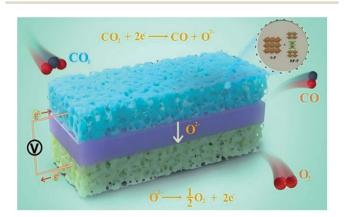
Scheme 1  $\,$  Schematic illustration of the cell configurations of SOECs for  $\mbox{CO}_2$  electrolysis.
