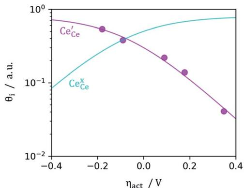
Fig. 4 Surface cation site coverage at the CGO–gas interface as a function of overpotential. Circles represent  $Ce'_{Ce}$  data collected by APXPS on a  $Sm_{0.2}Ce_{0.8}O_{1.9}$ –gas interface as a function of overpotential at 500 °C in 1 : 8 : 4  $H_2O$  :  $H_2$  : Ar atmospheres (Chueh *et al.*).<sup>16</sup> The fit for  $Ce'_{Ce}$  (magenta) and  $Ce^x_{Ce}$  (cyan) are found by solving eqn (11).
