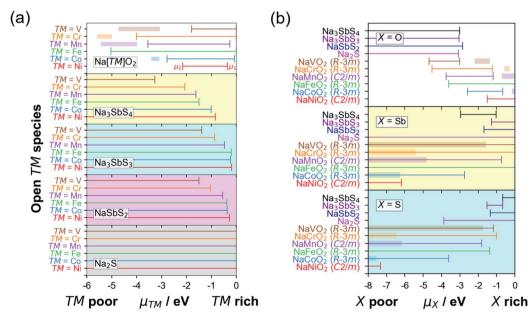
Fig. 3 (a) Chemical potential stability  $[\mu_1, \mu_2]$  range for TM species in Na[TM]O<sub>2</sub> (TM = {V, Cr, Mn, Fe, Co, Ni}) when in contact with t-Na<sub>3</sub>SbS<sub>4</sub> solid electrolyte (SE) and other sulfide-type SE-related phases. (b)  $[\mu_1,\mu_2]$  range for X species (X = {O, Sb, S}) for various Na[TM]O<sub>2</sub>-SE (SE-related) interface combinations. Horizontal bands are for same cathodes under charging condition (full desodiation).
