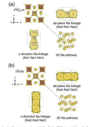
Fig. 1 (a) Crystal structure of t-Na<sub>3</sub>SbS<sub>4</sub> (P42<sub>1</sub>c) and (b) c-Na<sub>3</sub>SbS<sub>4</sub> (143m). Highlighted are Na atoms and isolated SbS<sub>4</sub> tetrahedral units, linkage of Na Wyckoff sites in the ab-plane, linkage of Na Wyckoff sites in the c-direction, and 3D perspective-view of the Na pathway.
