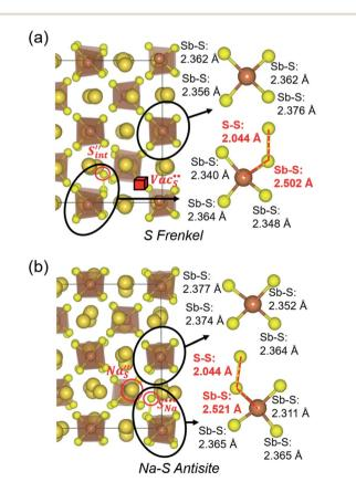
Fig. 7 Schematic illustration of (a) S Frenkel and (b) Na – S antisite from DFT-optimized supercells. Defect species such as  $S_{\rm int}^{"}$ ,  $Vac_{\rm S}^{"}$ ,  $Na_{\rm S}^{"}$ , and  $S_{\rm Na}^{"}$  and defect-related bond lengths are shown in red.
