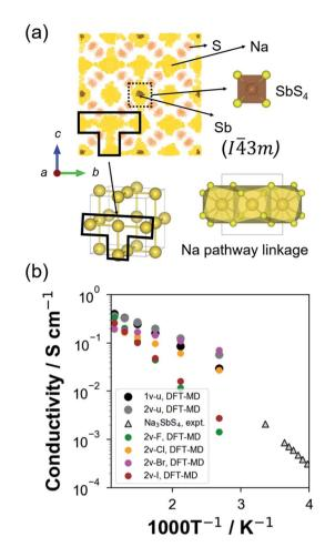
Fig. 8 (a) 2D-projected atom trajectory density from 100 ps NVT-MD calculation (473 K) of the 1-vacancy c-NSS (l43m) supercell model. (b) DFT-MD-derived Arrhenius plot for Na $^+$  ionic conductivity at different temperatures of 1-vacancy undoped (1v-u), 2-vacancy undoped (2v-u), F-doped (2v-F), Cl-doped (2v-Cl), Br-doped (2v-Br), and I-doped (2v-l) supercell models. Experimental data for undoped Na $_3$ SbS $_4$  are included for comparison.
