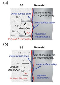
Fig. 5 Schematic illustration for conditions leading to (a) Na dendrite growth and (b) stable Na electrodeposition, based on the relationship between electron chemical potential ( $\mu_{\rm e}$ -) and surface roughness (wavenumber k) at the Na metal surface (peak and valley).
