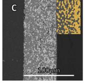
Fig. 1 Microstructure of the mixed cathodes from SEM images (a) thick cathode, (b) thin cathode, (c) gradient cathode.
