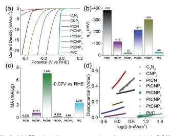
Fig. 5 (a) HER polarization curves on various electrocatalysts in 0.5 M  $\rm H_2SO_4$  at the rotation rate of 1600 rpm, potential sweep rate of 10 mV  $\rm s^{-1}$  and 85%  $\it iR$  compensation. (b) Corresponding  $\eta_{10}$  from the HER polarization curves in panel (a). (c) Mass activity at -0.07 V vs. RHE per  $\rm \mu g$  of Pt calculated from ICP-OES measurements. (d) Tafel plots derived from panel (a). Note the overlapping data points between the Pt/C and PtCNP2 samples.
