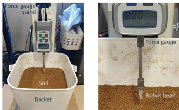
Fig. 8 Measurements of burrowing forces of the conical head.
