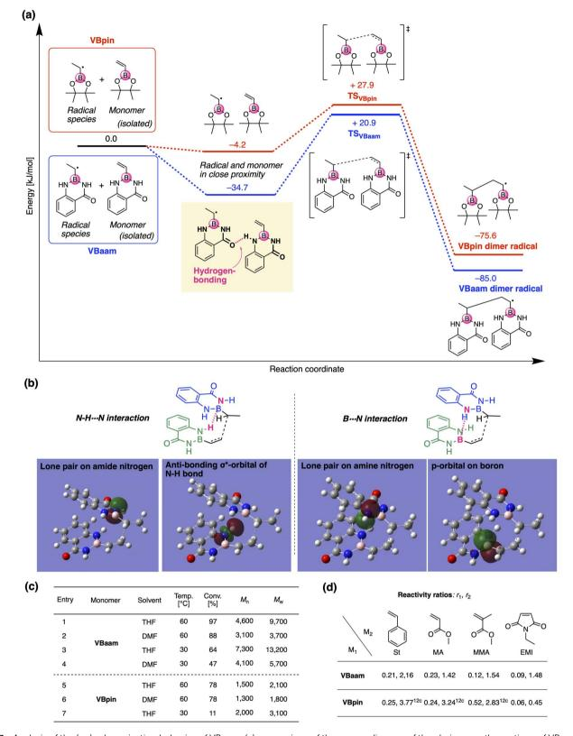
Fig. 3 Analysis of the (co)polymerization behavior of VBaam: (a) comparison of the energy diagram of the chain-growth reactions of VBaam and VBpin, calculated at the (U)CAM-B3LYP/6-31G(d) level. (b) Interactions between two aam groups observed in the NBO calculations. (c) Effect of the conditions on the polymerization of VBaam and VBpin. (d) Monomer reactivity ratios of the boron monomers  $(M_1)$  in copolymerizations with common vinyl monomers (M<sub>2</sub>) [ $r_1$  (left),  $r_2$  (right)].
