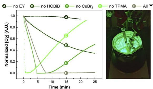
Fig. 5 Oxygen concentration measurements. Reaction conditions: [HOBiB]/[EYH<sub>2</sub>]/[CuBr<sub>2</sub>]/[TPMA] = 1/0.01/0.2/0.6, [HOBiB] = 1.5 mM, in PBS with DMSO (10% v/v), irradiated for 30 min under green LEDs (520 nm, 9.0 mW cm<sup>-2</sup>) in an open vial with stirring at 500 rpm.
