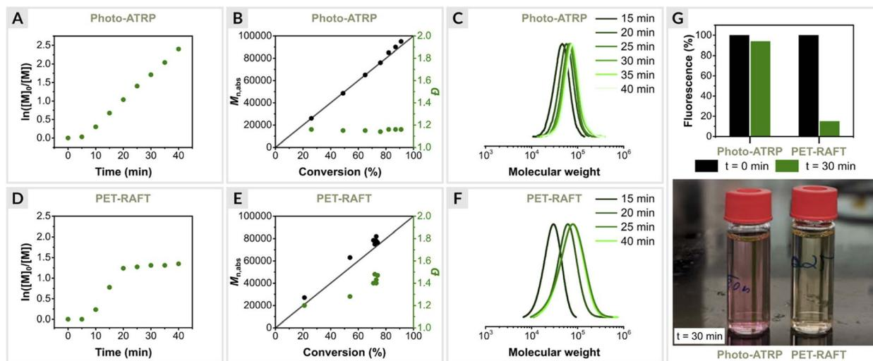
Fig. 3 Polymerization kinetics of OEOMA<sub>500</sub>. (A–C) EY/Cu mediated photo-ATRP and (D–F) EY-catalyzed PET-RAFT polymerization. (G) EY fluorescence intensity measurements.
