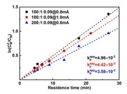
Fig. 4 First-order kinetic plot of different polymerization conditions.
