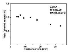
Fig. 8 Productivity of the reactor setup as a function of residence time.
