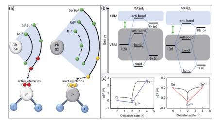
Fig. 1 (a) The electronic structure of Sn and Pb atoms. (b) Schematic energy levels of MASnl<sub>3</sub> vs. MAPbl<sub>3</sub> perovskites. (c) Frost diagrams of different oxidation states for Pb and Sn elements. <sup>47</sup> Copyright 2021, American Chemical Society.
