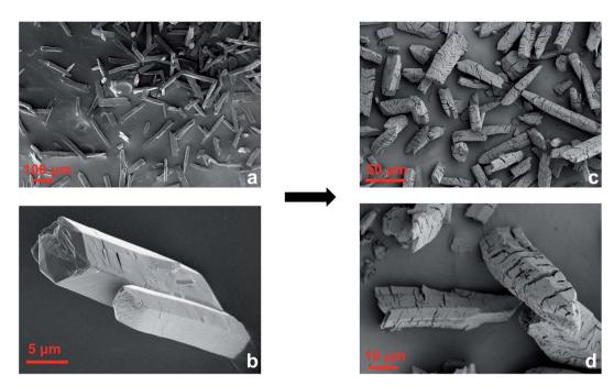
Fig. 3 SEM images of Cu-Sp5-BF<sub>4</sub>-A (a and b) and Cu-Sp5-OMe (c and d)
