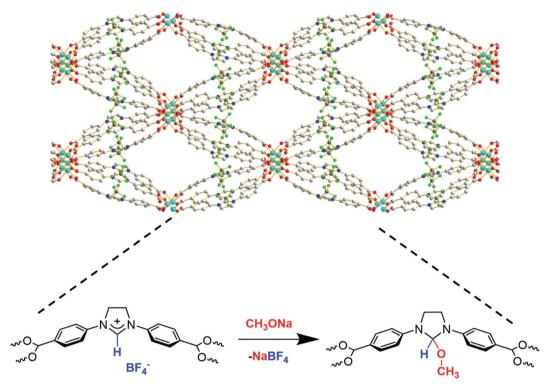
Scheme 1 Schematic of NHC-methoxide modification inside Cu-Sp5-BF₄-A.
