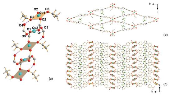
Fig. 1 Structure of Cu-Sp5-BF<sub>4</sub>-EtOH. (a) View of SBU, (b) view along the a axis depicting channel front, and (c) view along the c axis depicting walls of the channel and connection of SBUs with linkers. Hydrogen atoms on (b) and (c) are omitted for clarity. The hydrogen bond between O4 and O5 is highlighted in purple. Atom colors: C, gray; O, red; N, blue; H, white; B, brown; F, green; Cu, turquoise.
